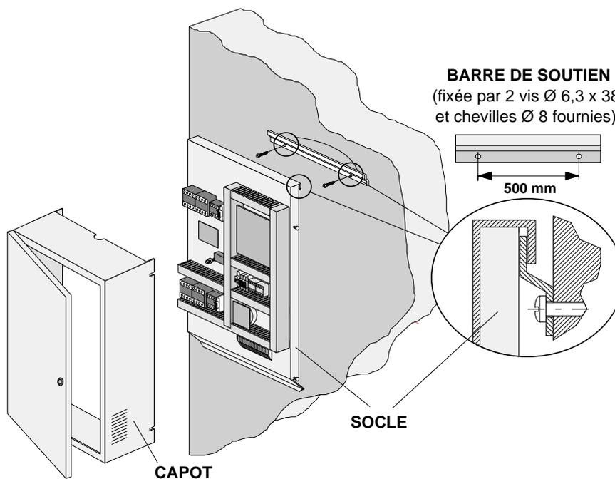
Dimensions de l'armoire Alpha Legend : L = 560 mm, H = 1000 mm, P = 250 mm
